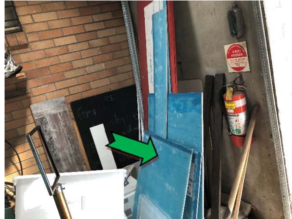
Photo 20. Interior, north elevation, garage/store, redundant panels – non asbestos-containing fibre cement sheeting.
